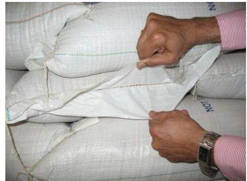
Photo no. 5: Gaps near Seams Large Enough for Insect Entry (Adama, Ethiopia)
