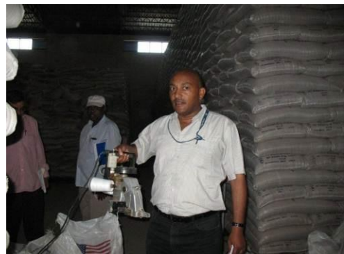
Photo no. 6: Poorly Lit Warehouse Interior (WFP, Adama, Ethiopia). A Handheld Machine for Stitching Torn Bags
