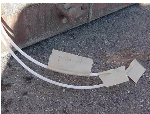
Gas Monitoring Lines
