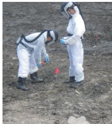
Collecting confirmation samples from the bottom of Sen Lake after excavation (Photo: CDM Smith)
