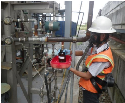
Collecting liquid samples from LVTP during thermal treatment operations (Photo: CDM Smith)
