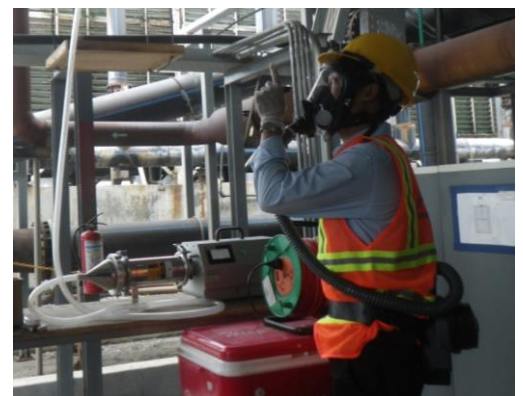
Chemical Command (Vietnamese Ministry of National Defense) collecting air samples in the liquid vapor treatment plant. (Photo: CDM Smith)
