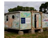
**Baylor College of Medicine** developed the Emergency Smart Pod, a portable, lightweight healthcare setting that can be expanded to a full-size unit in less than five minutes with just four people. In 2017, the Emergency Smart Pod was deployed to ELWA Hospital in Liberia, where it is used as an isolation unit for infectious patients.
