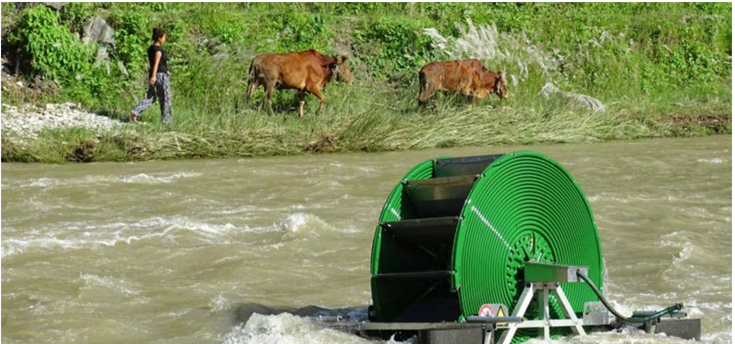
SWFF Grand Challenge Innovator aQysta's Barsha Pump runs on river currents alone and is, therefore, an environmentally friendly, low maintenance irrigation solution. Photo credit: aQysta
