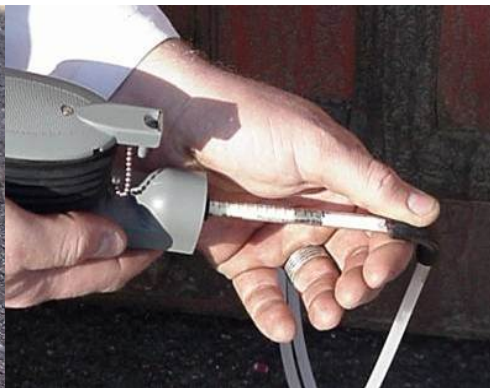
Gas Monitoring Line Connected to a Detector Tube
