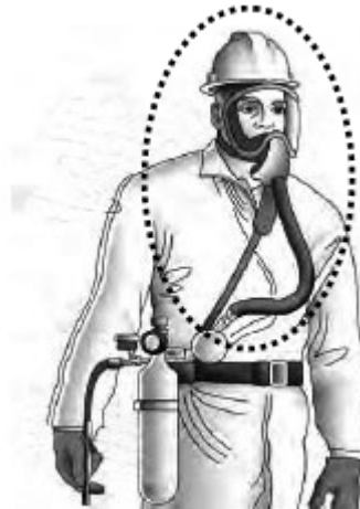
Supplied air respirator with full face mask
