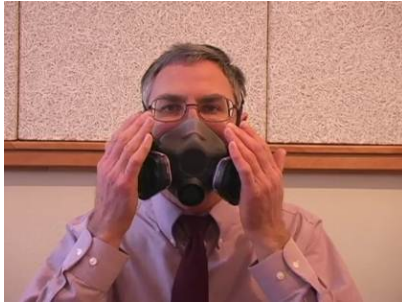
Fit Test for Cartridges to Determine Tight Fit
